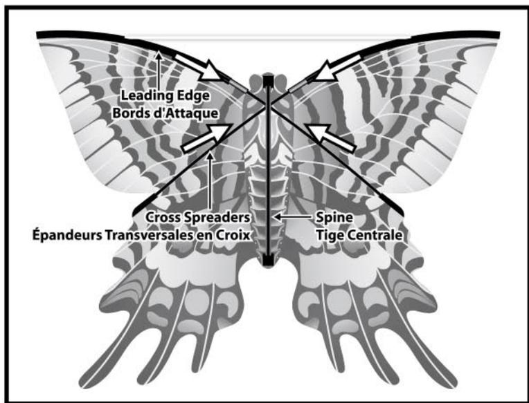
1. Connect Leading Edges and Cross Spreaders together. Be sure that Cross Spreaders pass beneath the Spine.
