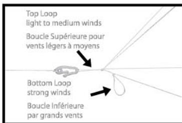
4. Attach the QuikClip® to the Bridle Loop. Top Loop for light to medium winds, Bottom Loop for strong wind.
